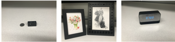
(a) Inconspicuous (b) Non-electrical camouflaged (c) Electrical camouflaged
